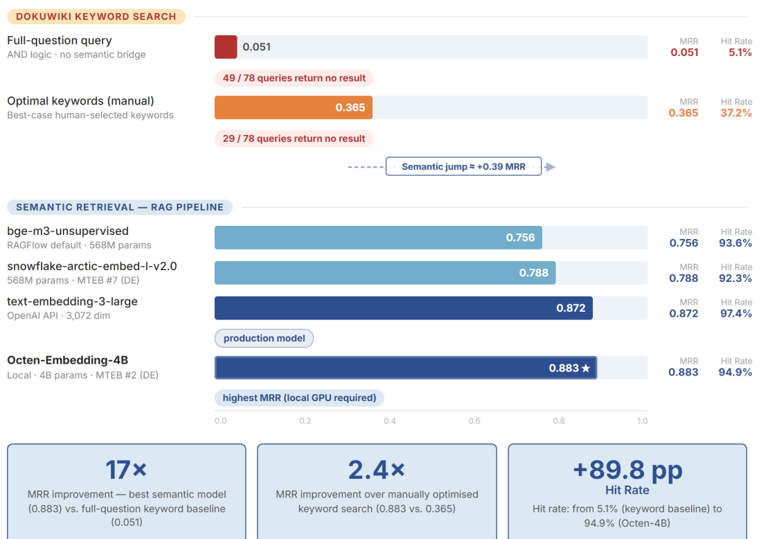
Figure 6.9: Overall comparison of DokuWiki keyword search vs. semantic RAG retrieval on 78 ground-truth questions. MRR bars are scaled to the full [0, 1] range across all evaluated retrieval methods.
