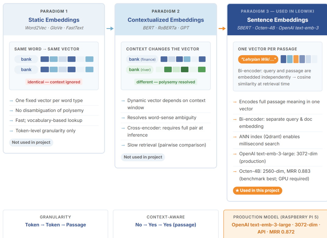
Figure 2.1: From token to sentence embeddings: static (Word2Vec), contextualized (BERT), and sentence-level (SBERT) paradigms. Sentence embeddings enable bi-encoder retrieval at scale.
