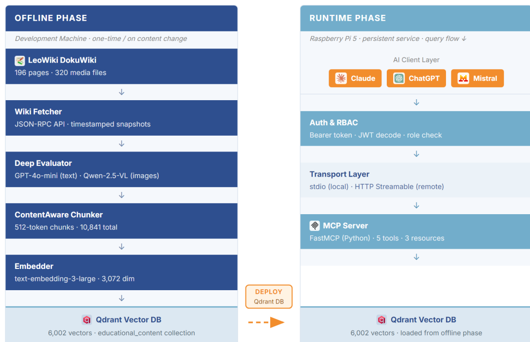
Figure 4.1: LeoWiki MCP system overview. The offline phase (left) prepares the knowledge base on a development machine: wiki content is fetched, evaluated, chunked, embedded, and indexed into Qdrant. The resulting vector database is deployed to the Raspberry Pi 5 (right), where the runtime phase serves semantic search queries via the MCP protocol to AI clients.
